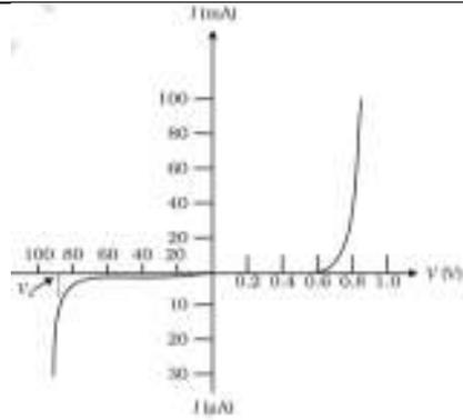
Beyond threshold voltage in forward bias diode current increases significantly even for very small increases in diode bias voltage.
